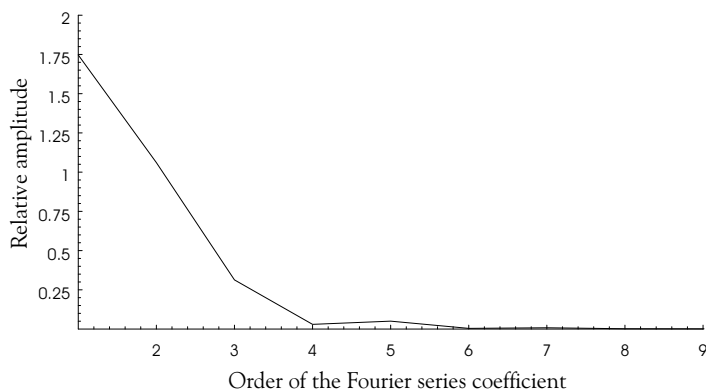
Fig. 4. Amplitude of Fourier coefficients in the first fluid-fluid interface case.
