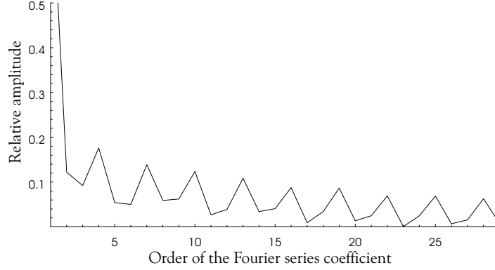
Fig. 8. Amplitude of Fourier coefficients in the fluid-solid interface case.
